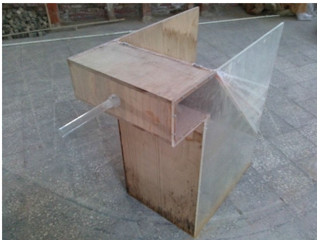
Fig. 3 OWC system with a width of 50 cm
