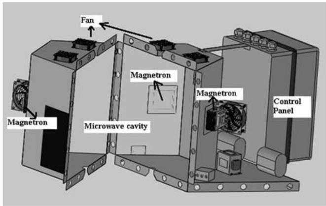
Fig. 2. Schematically illustration of microwave oven
