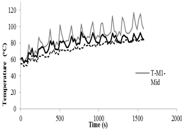
**Fig.4.** Variation of temperature along the adsorbent bed across the magnetron 1.
