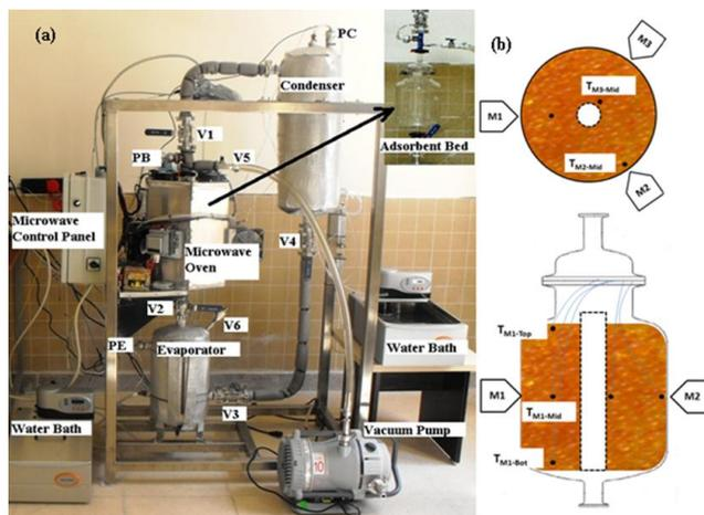
**Fig.1a.** Photograph of the designed intermittent adsorption heat pump, **b.** Location of thermocouples in the adsorbent bed.
