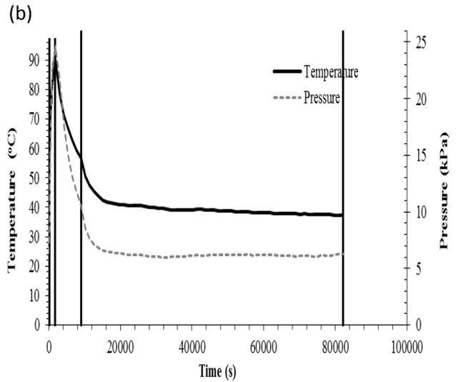
**Fig.5.** Variations of bed temperature and pressure during all cycle process for a) Conventional heating b) Microwave heating
