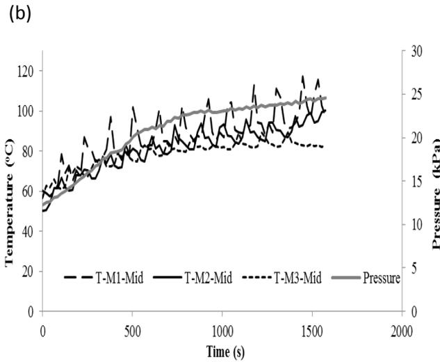
**Fig. 3.** Adsorbent bed temperature and pressure during isobaric desorption process for a) Conventional heating system b) Microwave heating system
