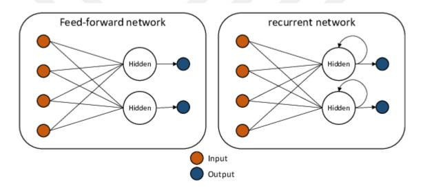
Figure 4. RNN with the characteristic cyclical connectivity. [4]
