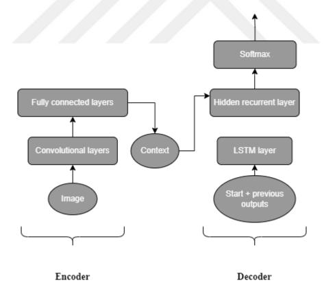
**Figure 8.** Architecture for image captioning network (encoder – decoder network
