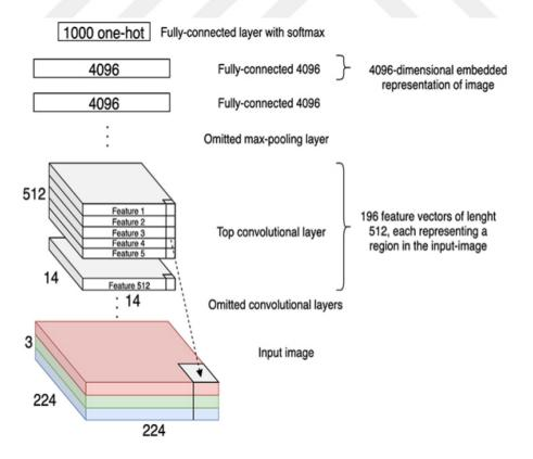
Figure 7. Simplified view of the VGG19 network where many layers have been omitted [5]
