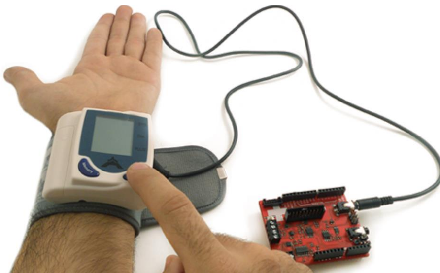
Figure. 37 D Blood pressure sensor connection
