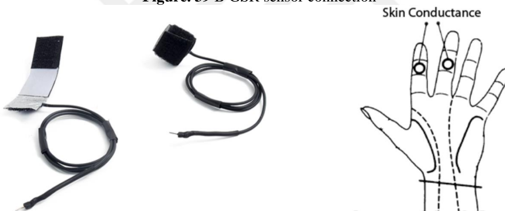
Figure. 39 B GSR sensor connection
