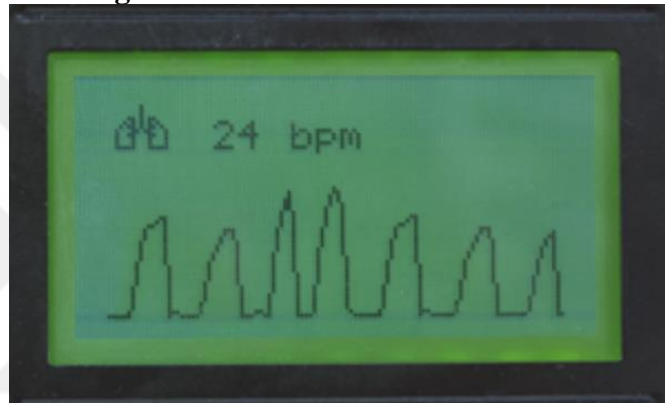
Figure. 78 Airflow wave in GLCD Test - Breathing measure
